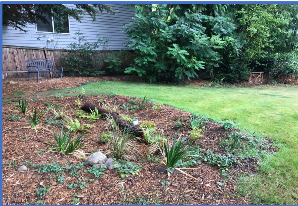
A rain garden manages water from 1000 square feet of roof area.
