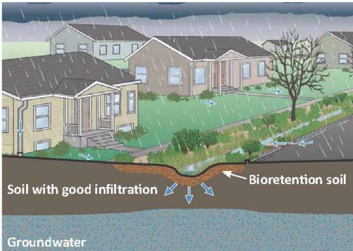
Image Bioretention with shallow infiltration (no underdrain) in planting strip. Graphic from WTD Barton project outreach materials.
