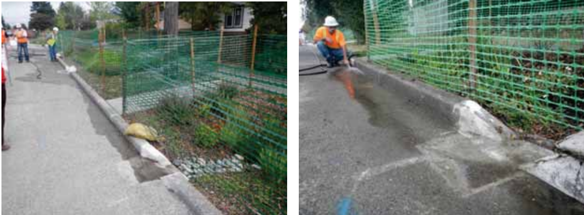
Images: Examples of gutter flow test for COS Std Plan 295b Drain Curb Cut Type 1.
