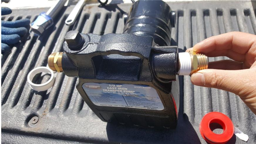
3. Now it's time to attach the hose from the inlet of the pump to the spigot of the cistern. Besure to use sealant putty or tape whenever there is an attachment involving threads.
